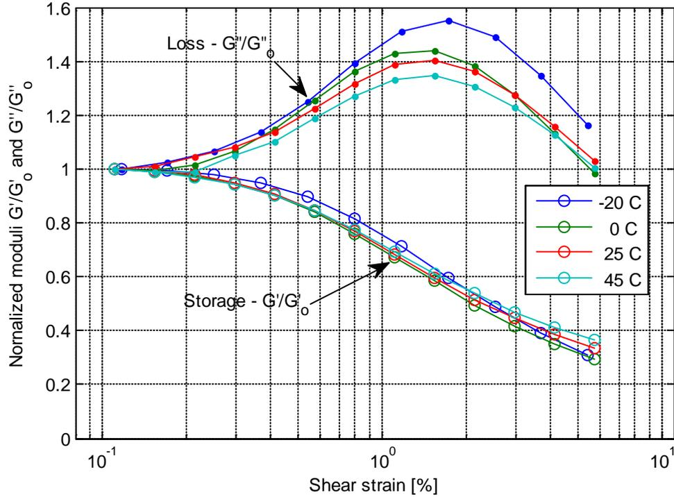
Fig. 6: Storage and loss moduli data normalized to the small strain values.
