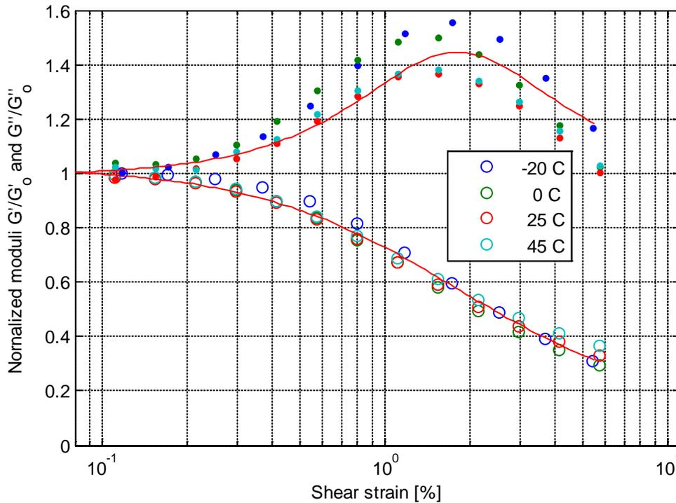
Fig. 7: Normalized storage and loss moduli with curve fits.
