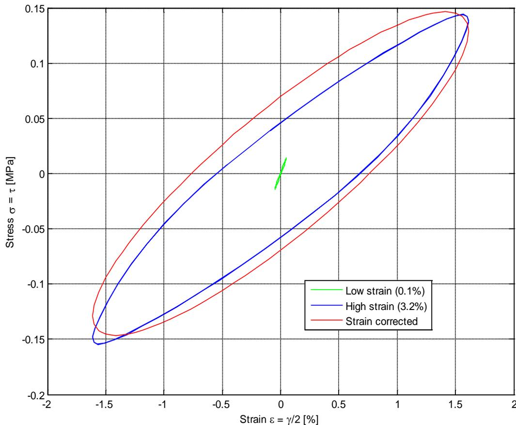
Fig. 8: Stress/strain cycles for low and high amplitude strains
