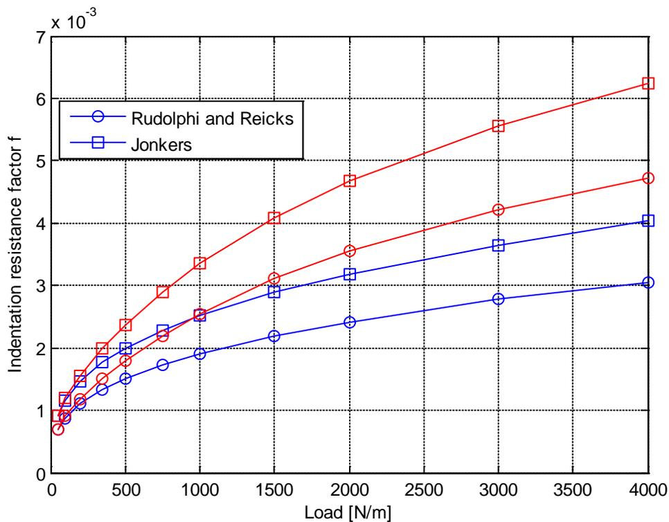
Fig. 9: Indentation resistance factors for small strain and strain-adjusted properties.
