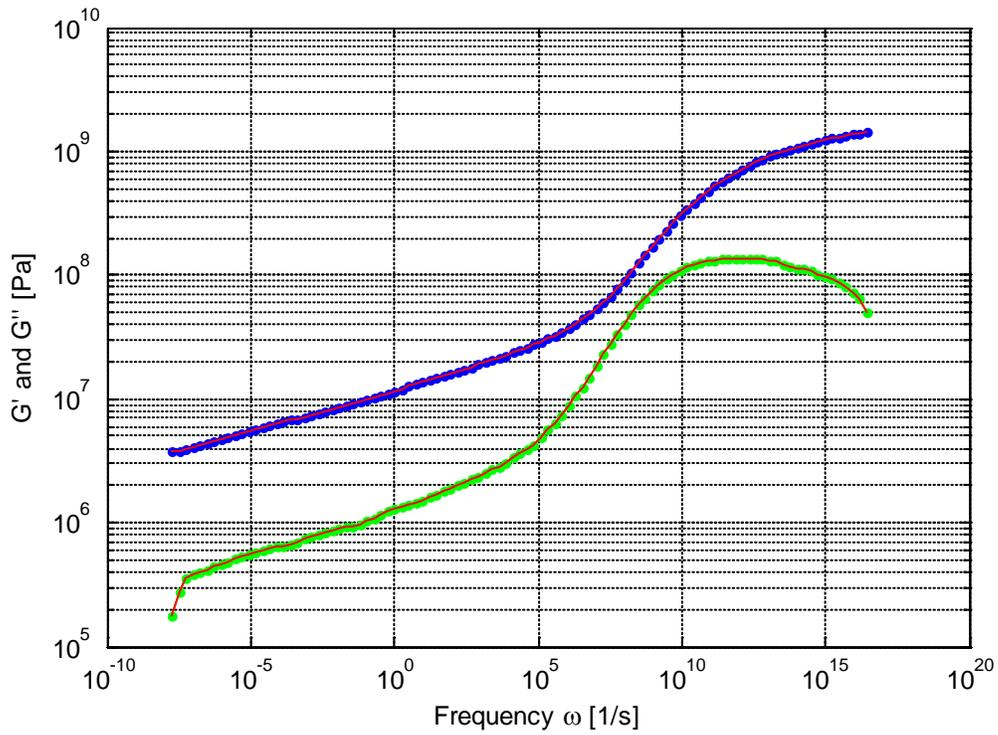
Fig. 2: Master curve of the shifted data and Prony series (spectral) fit to the shifted data.
