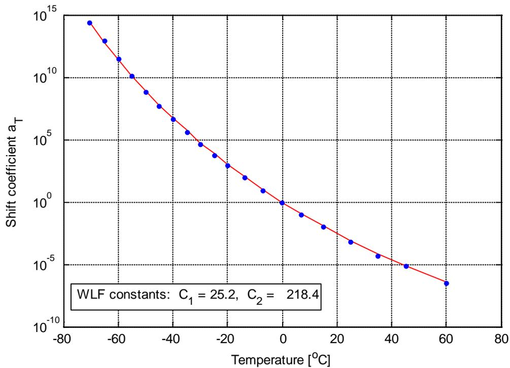
Fig. 3: Frequency-temperature shift coefficient  $a_T$  and WLF curve fit.
