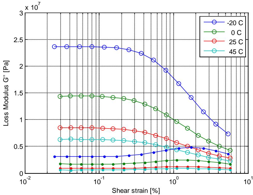
Fig. 5: Storage and loss moduli data at various temperatures.
