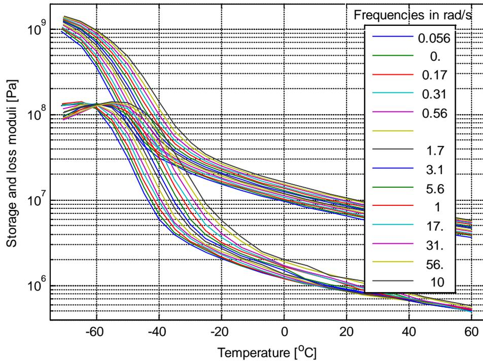
Fig. 1: Storage and loss moduli data for temperatures and frequencies tested.
