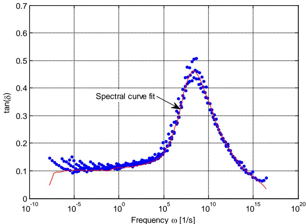
Fig. 4: Loss tangent and spectral representation of the data.
