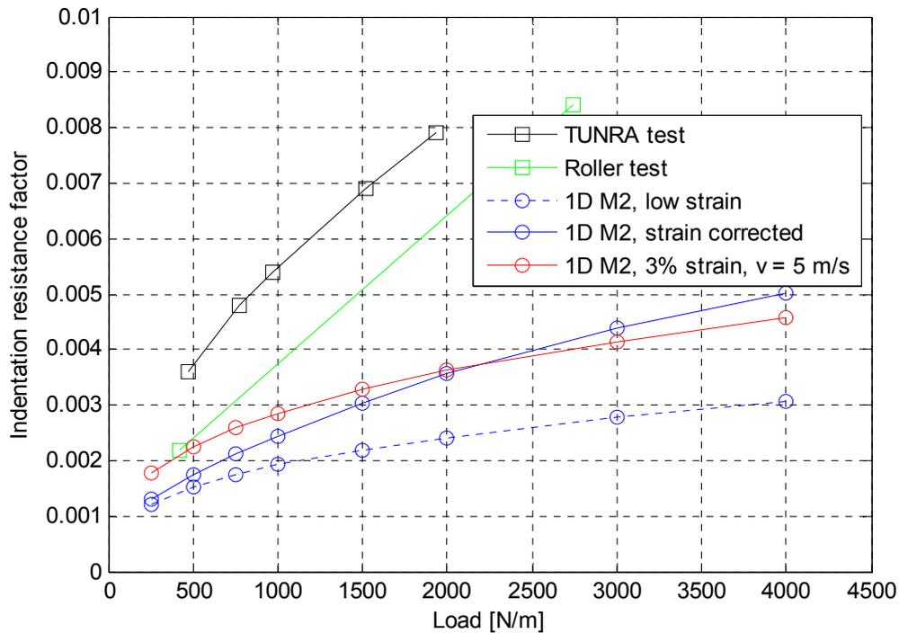
Fig. 5: Indentation resistance factor - measured and calculated - at various loads.
