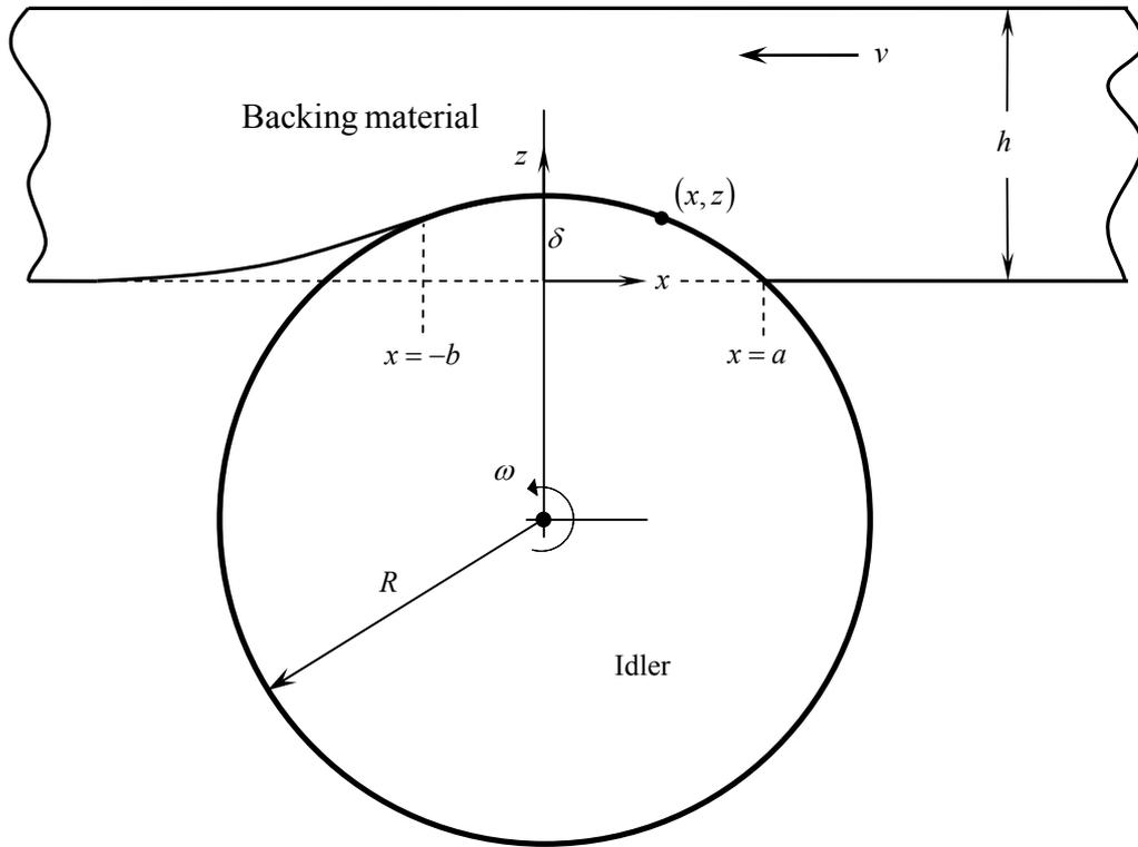
Fig. 1: Schematic of viscoelastic behavior during belt cover indentation
