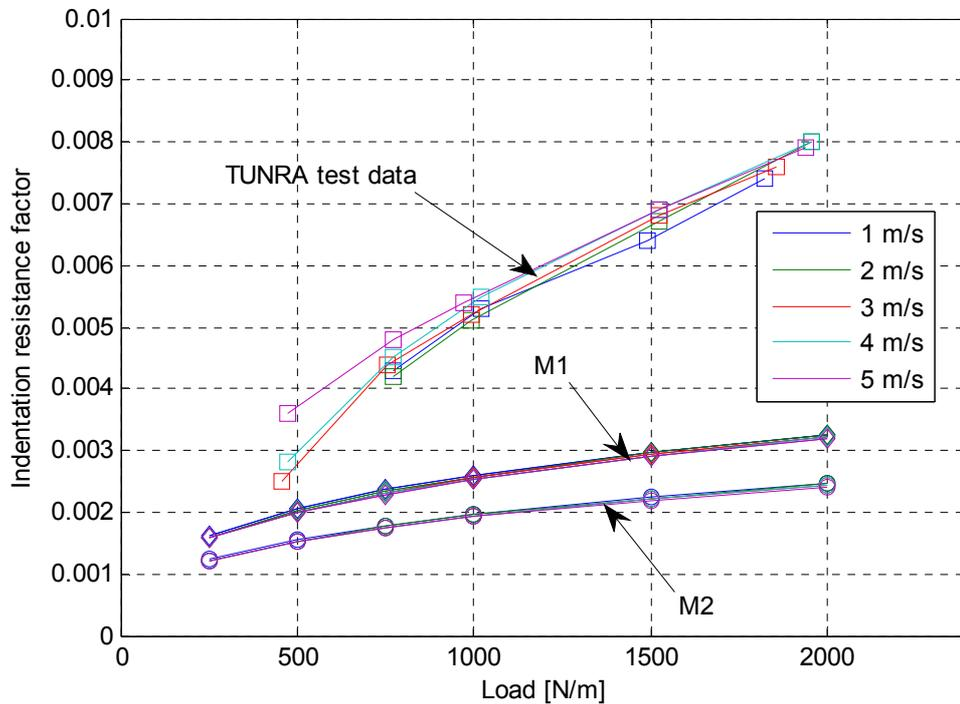
Fig. 4: Indentation resistance at low strain and various belt speeds.
