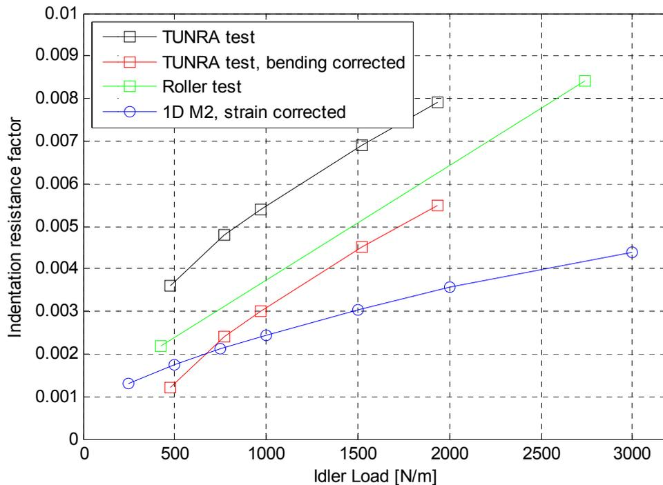
Fig. 6: Indentation resistance factor - calculated, measured and bending loss corrected.
