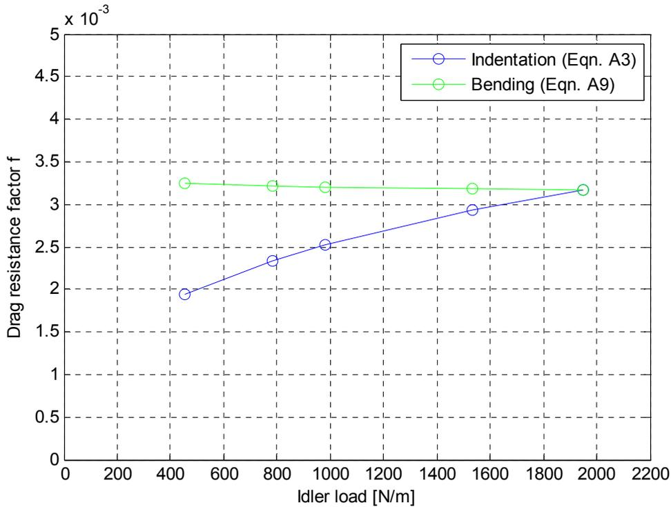
Fig. A1: Drag resistance factor for indentation and bending by energy dissipation.
