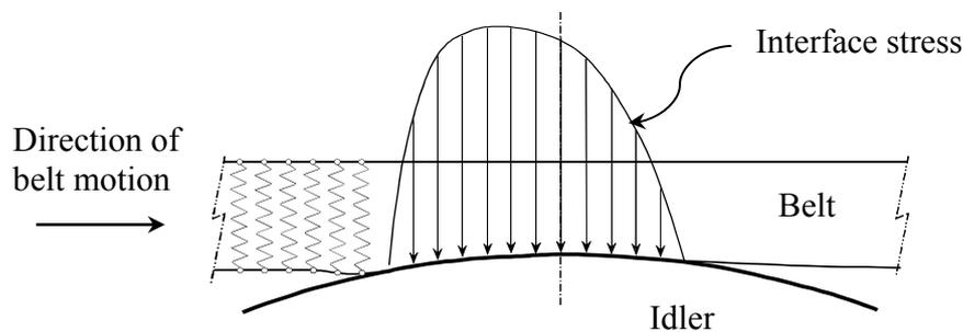
Fig. 2: Winkler representation of the indentation and stress between the belt and idler.
