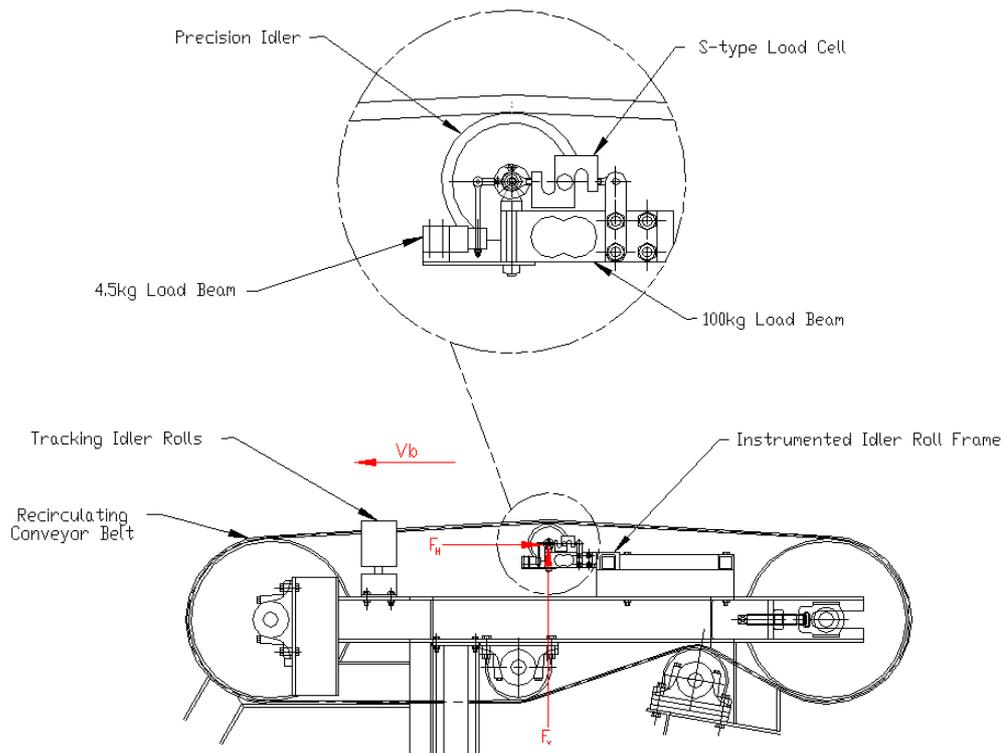
Fig. 3: Illustration of the TUNRA Bulk Solids conveyor belt indentation rolling resistance test facility.
